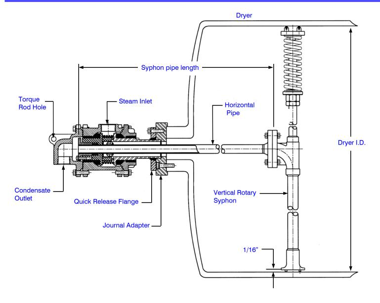
The Barco Rotary Syphon is designed specifically for use in condensate removal systems for paper machine dryers.
